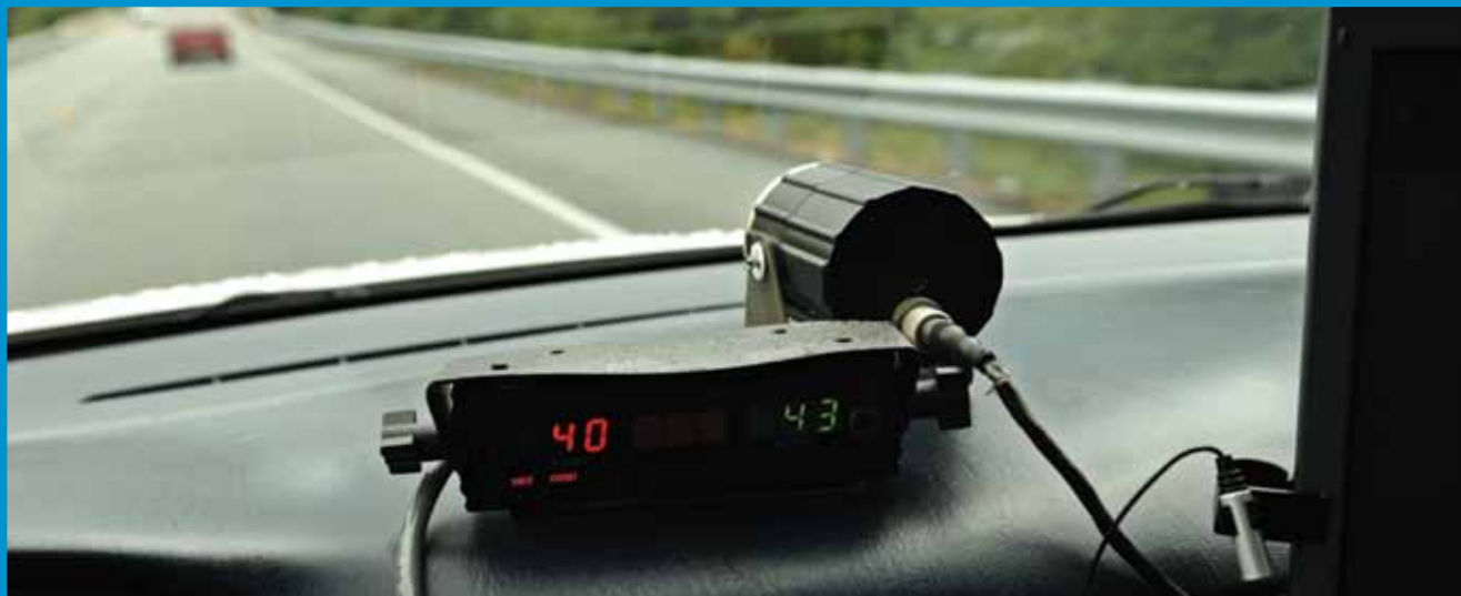
GTSI's Mobile Evidence Capture solution includes syncing radar with in-dash laptop to record traffic data.
